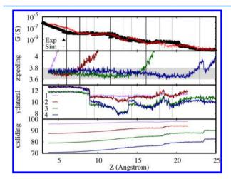
**Figure 3.** Peeling (z), lateral (y), and sliding (x) motions of the center of mass of the four terminal fluorene units (1-4) of the PF chain during the pulling. As a reference, the conductance–distance profile is included in the upper panel.
