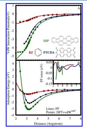
**Figure 1.** Force field (FF) for molecule–metal interactions. (A) vdWs and (B) net adsorption interactions for benzene (BZ), diindenoperylene (DIP), and perylene-3,4,9,10-tetracarboxylic dianhydrid (PTCDA) on Au(111) as a function of the molecule–surface distance. The Figure compares the FF (lines) with DFT + vdW<sup>surf</sup> adsorption (dots) curves when the molecules are parallel to the surface. The inset shows the net FF errors.
