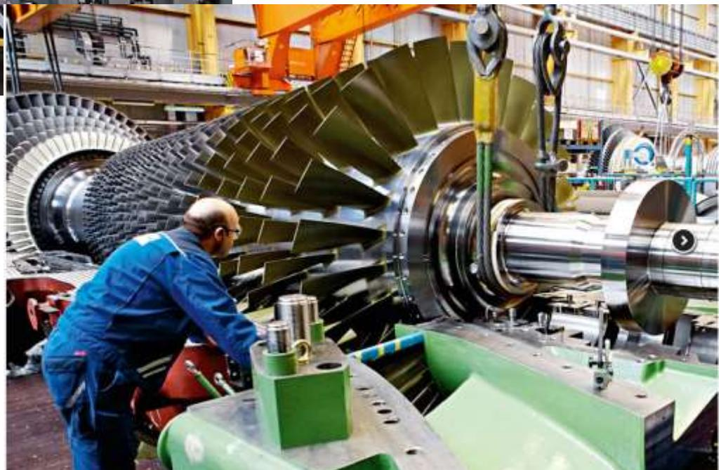
Available for different power outputs (5-375 MW), revolutions 3,000-17,000 rpm, 50/60 Hz electric.
