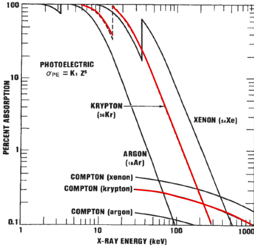
Relative absorption of various proportional counter gases for low energy x-rays (Taken from Reference 1).
