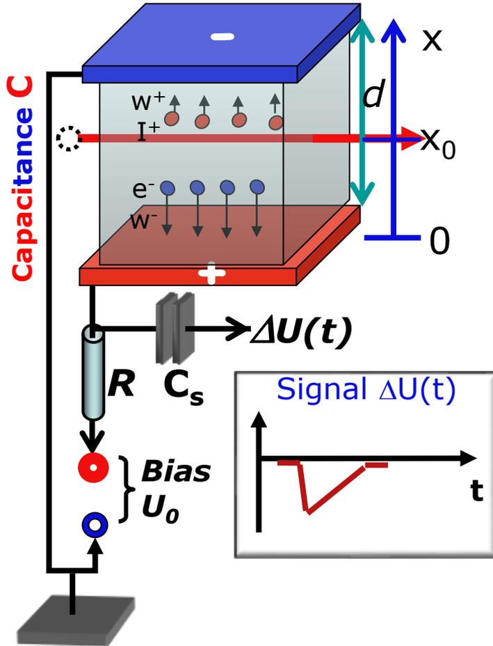
Energy loss  $\Delta\varepsilon$ :  $n = n_I = n_e = \Delta\varepsilon/I$  number of  $n$  primary ion pairs ( $I^+, e^-$ ) at  $x_0, t_0$
