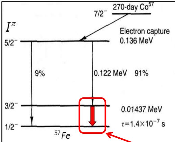
Measure very small differences in  $3/2^- \rightarrow 1/2^-$  transition energy depending on differences of environments of  $^{57}\text{Fe}$  nuclei embedded in source and absorber.
