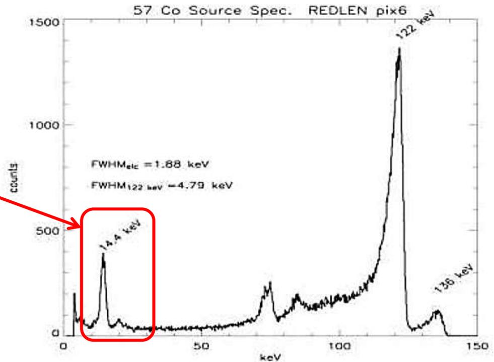
Measurement with CdZnTe (CZT) solid-state detector.
