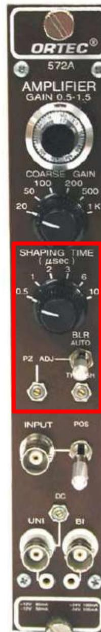
**Tasks:** Generate signal with amplitude **proportional** to collected detector charge. Needs absolute calibration of pulse amplitude.
