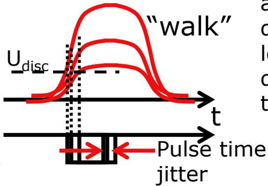
amplitude dependent leading edge discr. output timing
