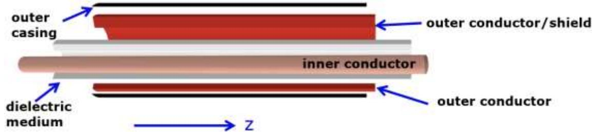
Coaxial cables/transmission lines  $\leftrightarrow$  traveling waves in cavity resonators
