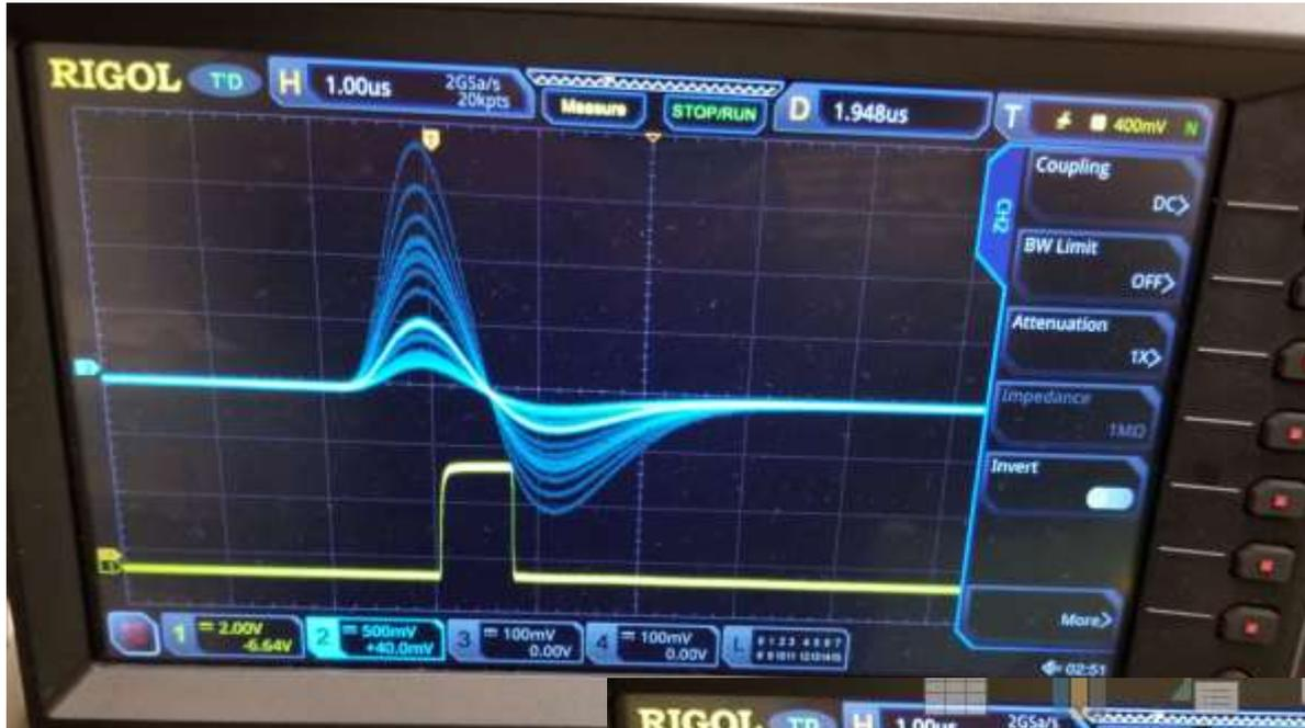
For triggering the ANSEL DDC-8 DAQ units, use the **negative** TSCA output signal ("NIM-0 In")
