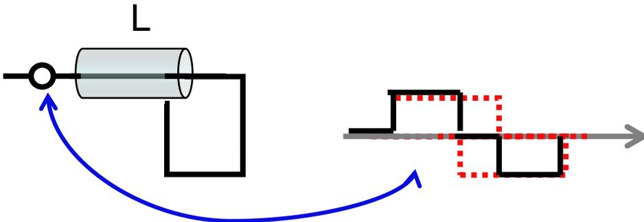
Short:  $R_{load} = 0$ , Input and reflection opposite polarity, superposition = bipolar
