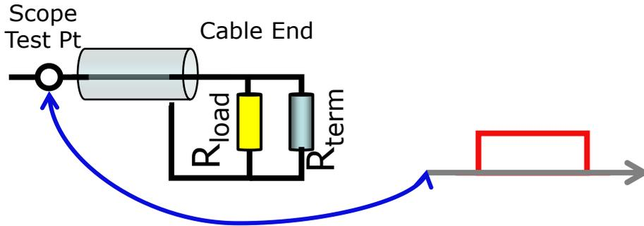
Receiver input impedance  $R_{load} \neq Z_0$ ,
