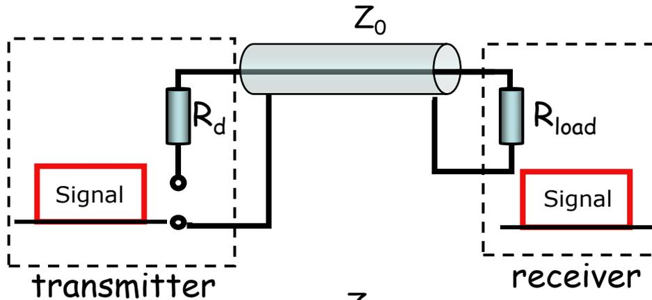
Coax cable has complex impedance  $Z$  for signal transmission,  $\text{Re}Z = Z_0$
