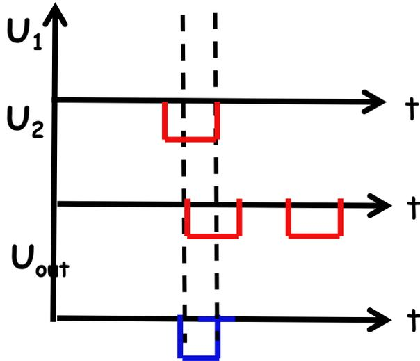
For fast timing: use fast negative logic
