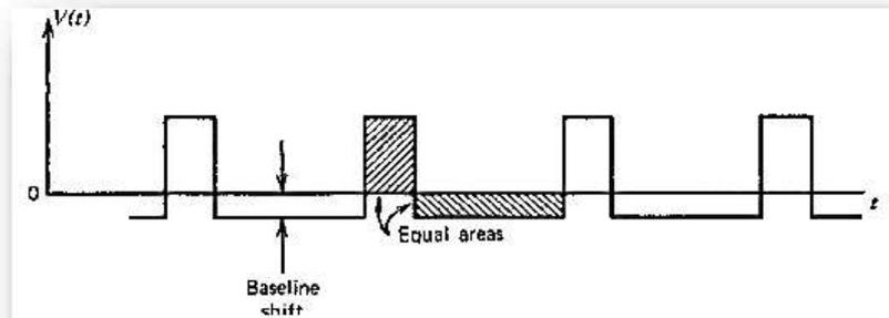
Preamplifier uncorrected base line shift
