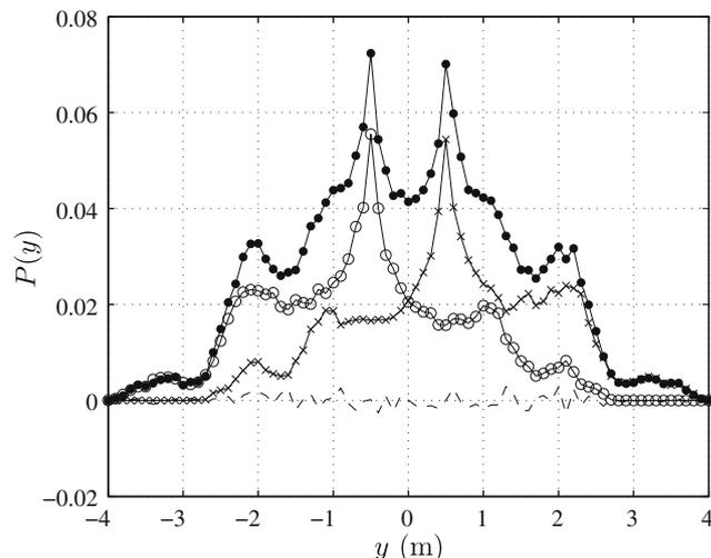
**Fig. 2.** Probability density distribution at the detection screen of the double-slit experiment schematically shown in Fig. 1 after launching 300,000 particles. The  $\bullet$ 's correspond to the case in which the two slits are open. The  $\circ$ 's and  $\times$ 's to the one in which only the lower or upper slit is open, respectively. The broken line represents the classical interferences in the observable  $P_{12}^c(y)$ .
