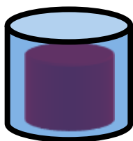
Fig. III-1a: Iso- lated system. No mass or heat ex- change
