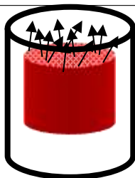
Fig. III-1c: Open system. Mass and heat exchange
